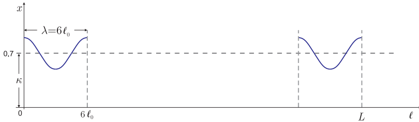
Figure 5. The one-dimensional space distribution of reactant activator x = x_0 + A \cos(q\xi) for the mode with \lambda = 6\ell_0 , where \ell_0 = \sqrt{Dt} is the characteristic diffusion length. x_0 = \kappa = 0.7 , A = 0.05 , L = 3\ell_0 n . The amplitude is exaggerated in order to be easily noticeable. The dot line is the steady-state level of the concentration of X .
