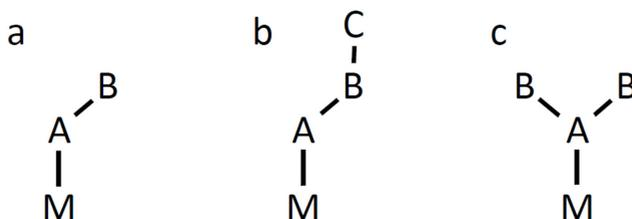
**Figure 1.** Three typical ligand moieties: an AB ligand in a bent form (a), a bent ABC ligand in a bent form (b), and a  $C_{2v}$ -symmetric  $AB_2$  ligand (c).
