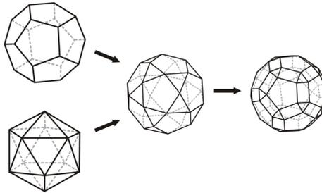
Figure 12: The dodecahedron and the icosahedron are half-truncated twice into the rhombicosidodecahedron.
