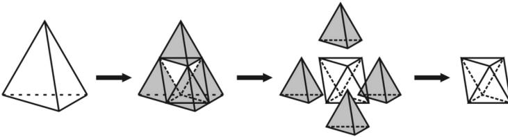
Figure 5: The tetrahedron is half-truncated into the octahedron.
