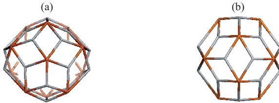
Figure 2. Bipartite, partial cubes: (a) five fold and (b) two fold symmetry, of the cage designed by sequence Du(Med(D)) : v=32 ; e=60 ; f_4=30 ; \Omega(G, x) = 6X^{10} ; \Pi(G, X) = 60X^{50} ; CI(G) = \Pi(G) = 3000
