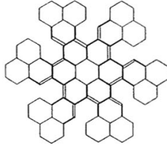
Figure 1.2: A hexagonal system with seven normal components. (Heavy lines indicate fixed single edges and double lines indicate fixed double edges).
