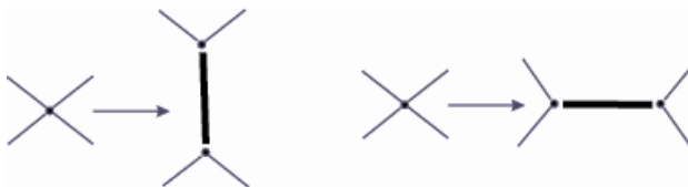
Figure 1. Two ways of the operation of vertex bifurcation (bigons are denoted by bold edges).
