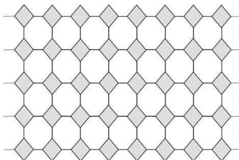
Figure 1- The  $TUC_4C_8(R)$  Nanotube with  $p=8$  and  $q=5$
